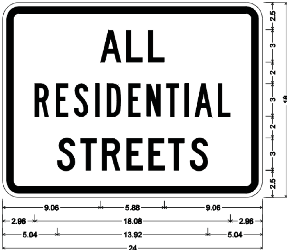
R2-20-24; 1.50" Radius, 0.63" Border, 0.38" Indent, Black on White; [ALL] C; [RESIDENTIAL] B 125% spacing; [STREETS] C; Table of distances between letter and object lefts.
