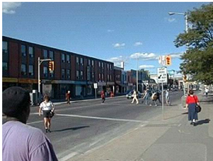
Figure 17. Pedestrian-Actuated Mid-block Signal. From www.pedbikeimages.org / ITE Pedestrian Bicycle Council. Reprinted with permission.
