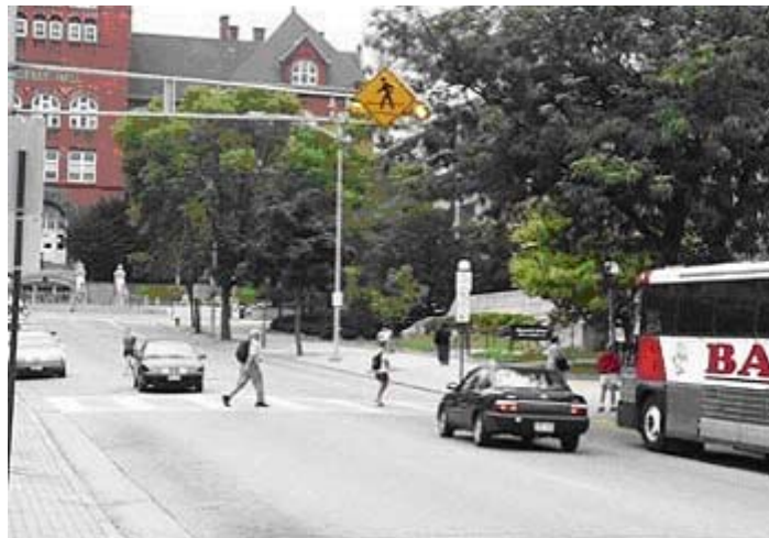
Figure 14. Overhead Sign with Flashing Beacons. From www.pedbikeimages.org/ ITE Pedestrian Bicycle Council. Reprinted with permission.
