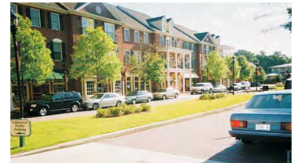
On-street parking and median divided streets are an alternate public street system to be considered for applicable design concepts such as neo-traditional and new urbanism development.
