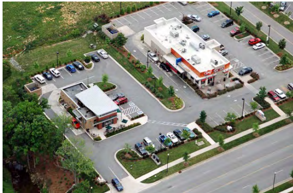
Retail buildings with connected parking lots to decrease entrance points on the main road
