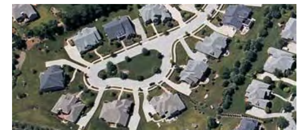
Islands in cul-de-sacs can create turning movement problems and parking opportunities that inhibit service delivery capabilities.
